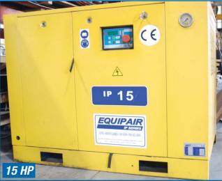
**EQUIPAIR ROTARY SCREW AIR COMPRESSOR**
